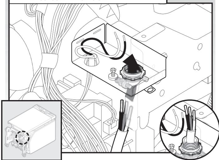
Route cord so that it does not touch dishwasher motor to lower part of dishwasher tub. Pull cord through strain relief in terminal bow.
